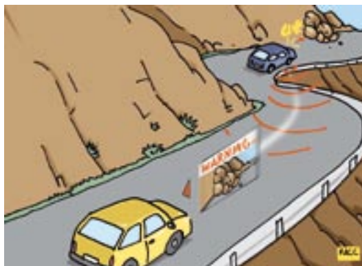
Vehicle-to-vehicle communication: The passenger car damaged by falling rocks alerts approaching vehicles to the potential danger.
